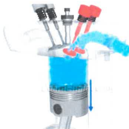
Figura 4.8. Admisia la motoarele Diesel (Sursa: Learn Engineering).
