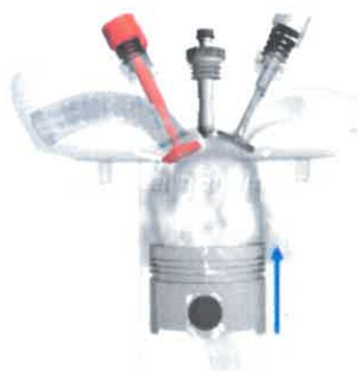
Figura 4.11. Evacuarea la motoarele Diesel (Sursa: Learn Engineering).
