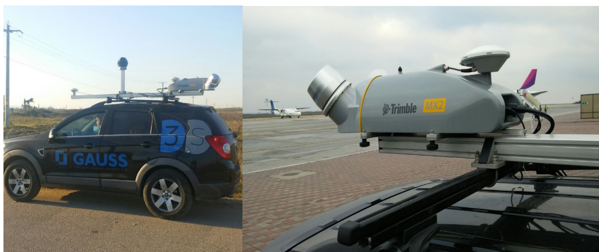
Figura 2 - Scanner-ul Trimble SLM – 250
